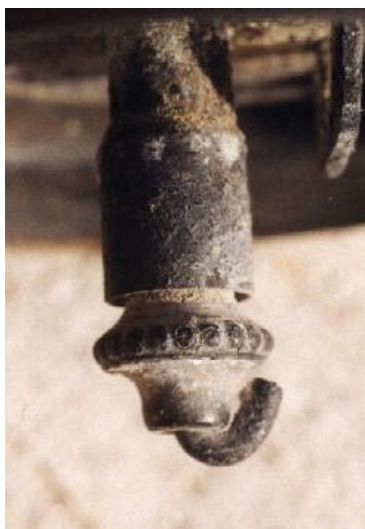
Duplex Feed as on pre-1920 lamps.
