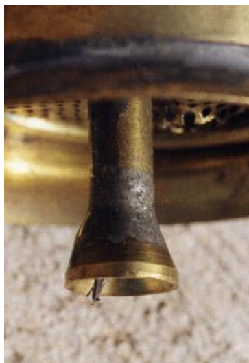
Inverted cone feed as on Platypus lamp.
