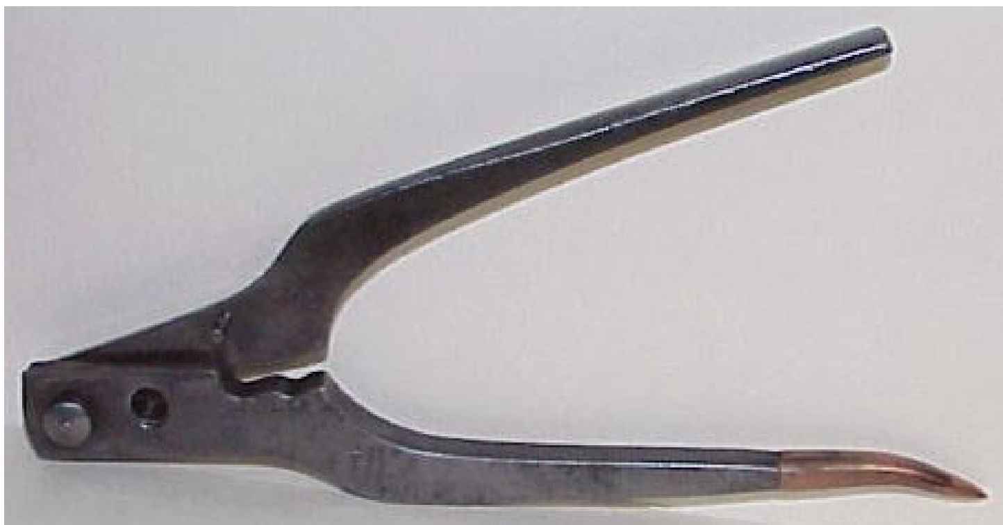
The Boker tool in the open position. Note the copper punch on the lower handle.
